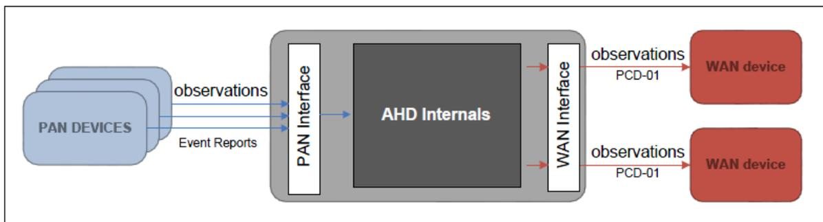
**Figure 42 : Model showing how AHD may collect observations from multiple PAN devices at any given point in time and a single PAN device may deliver data to multiple persistent sessions. Likewise, an AHD may deliver these observations to zero or more WAN devices.**
