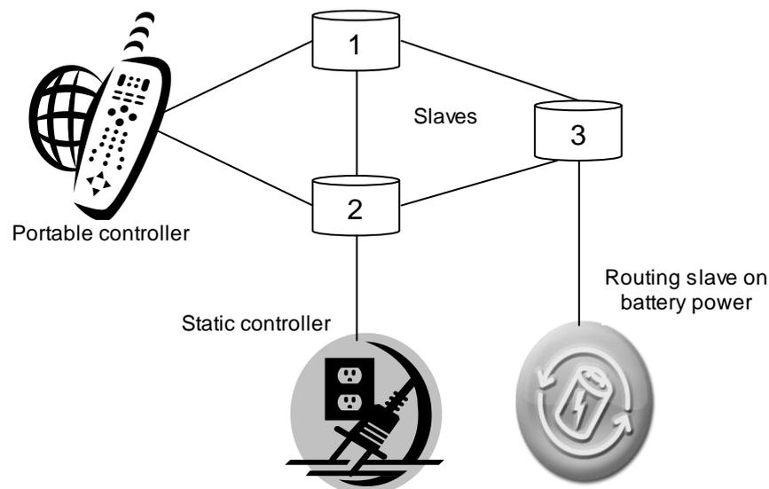
Figure 10 : Z-Wave topology with control devices and slave nodes
