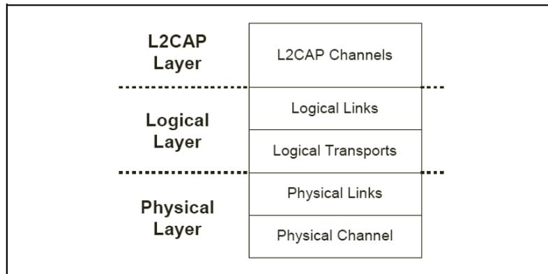
Figure 4 : Bluetooth generic data transport architecture
