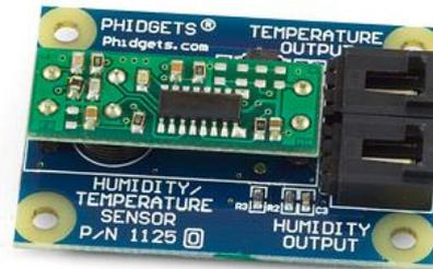
**Figure 30 : Phidget humidity and temperature sensor.**
