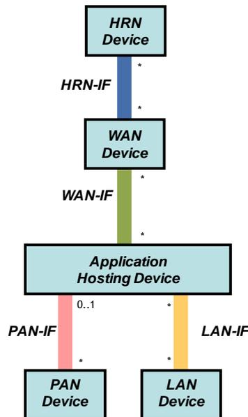
**Figure 43 : Continua Topology (from Continua Design Guidelines V1.5)**
