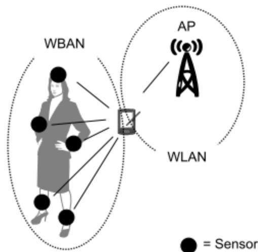
Figure 13 : Extending WBAN range using WLAN
