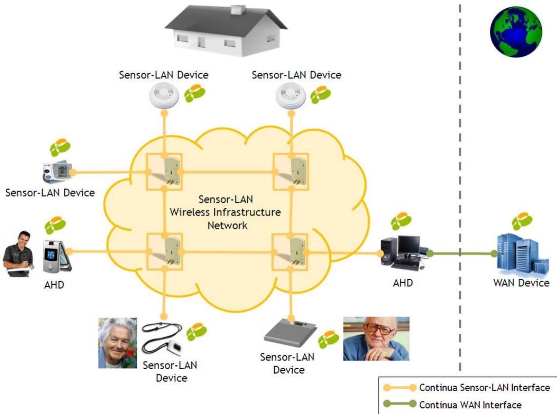
**Figure 41 : Sensor-LAN Conceptual Setup (from Continua Sensor LAN Interface Design Guidelines)**
