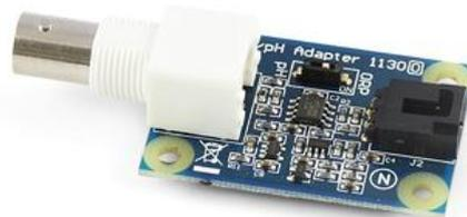
**Figure 29 : pH/ORP phidget sensor adapter.**
