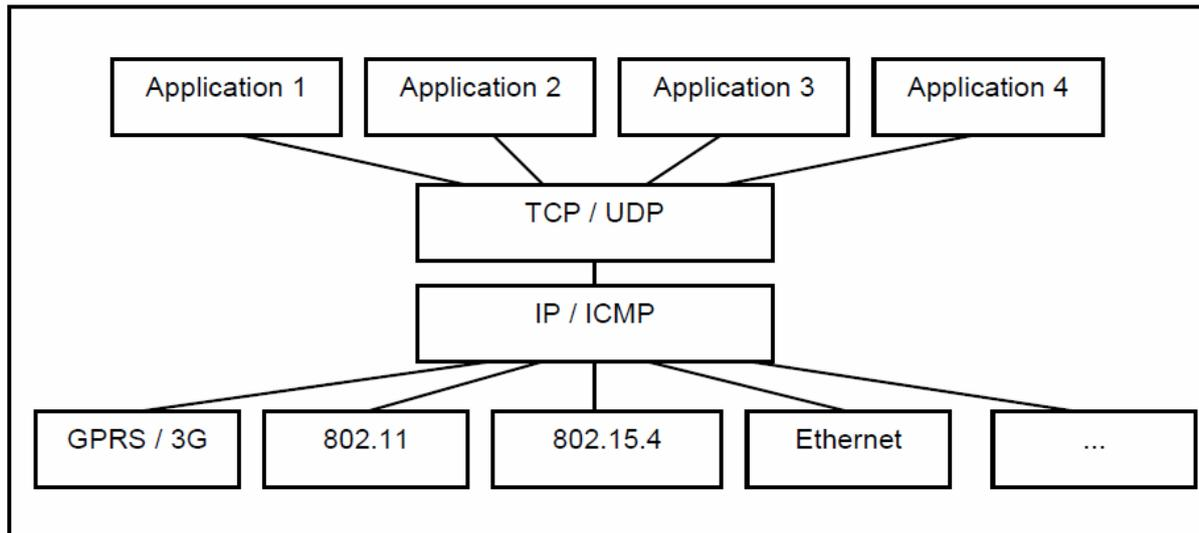
**Figure 33 : IPv6 layered architecture with communication flexibility<sup>21</sup>.**
