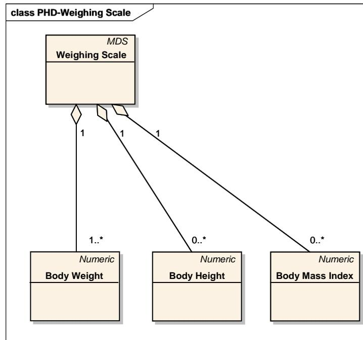
**Figure 40 : Object model for Weighing Scale following IEEE 11073-10415:2008**
