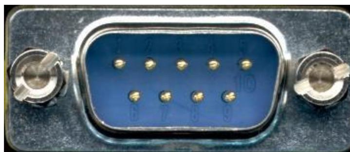
**Figure 20 : D-sub 9 connector pinout**
