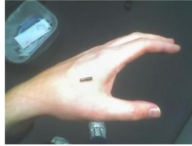
**RFID tag for implant into human hand**
