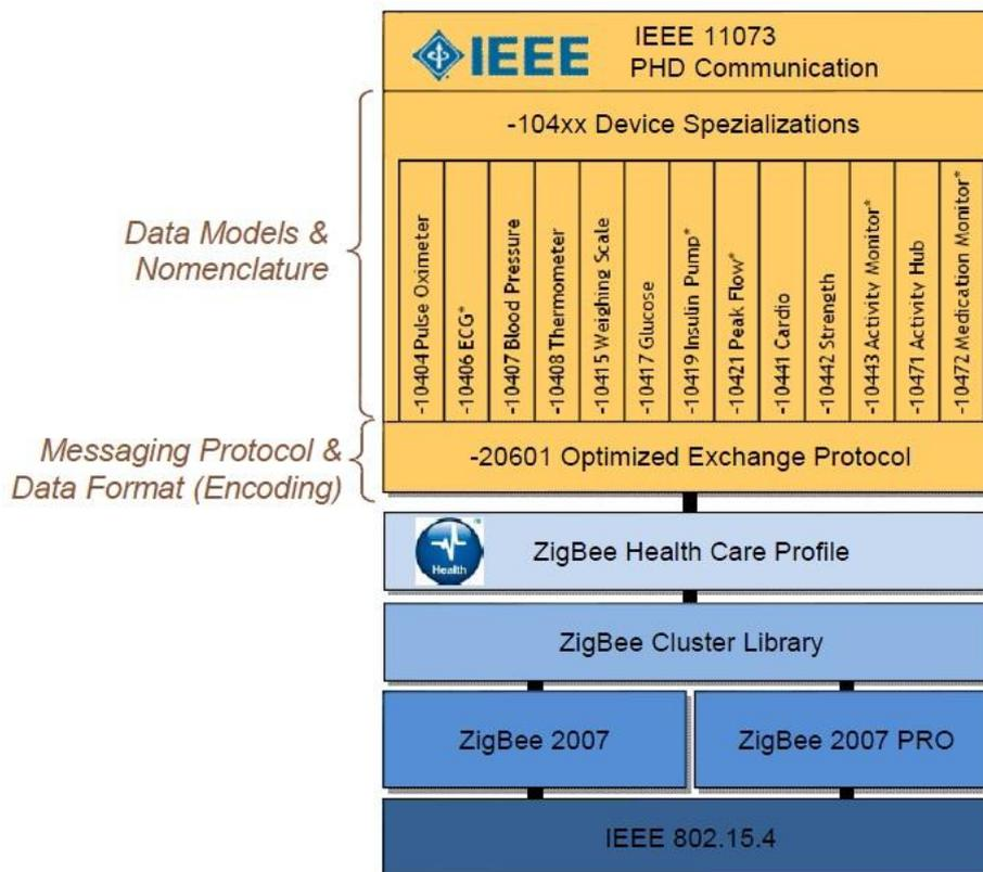
**Figure 9 : ZigBee Health Care architecture**
