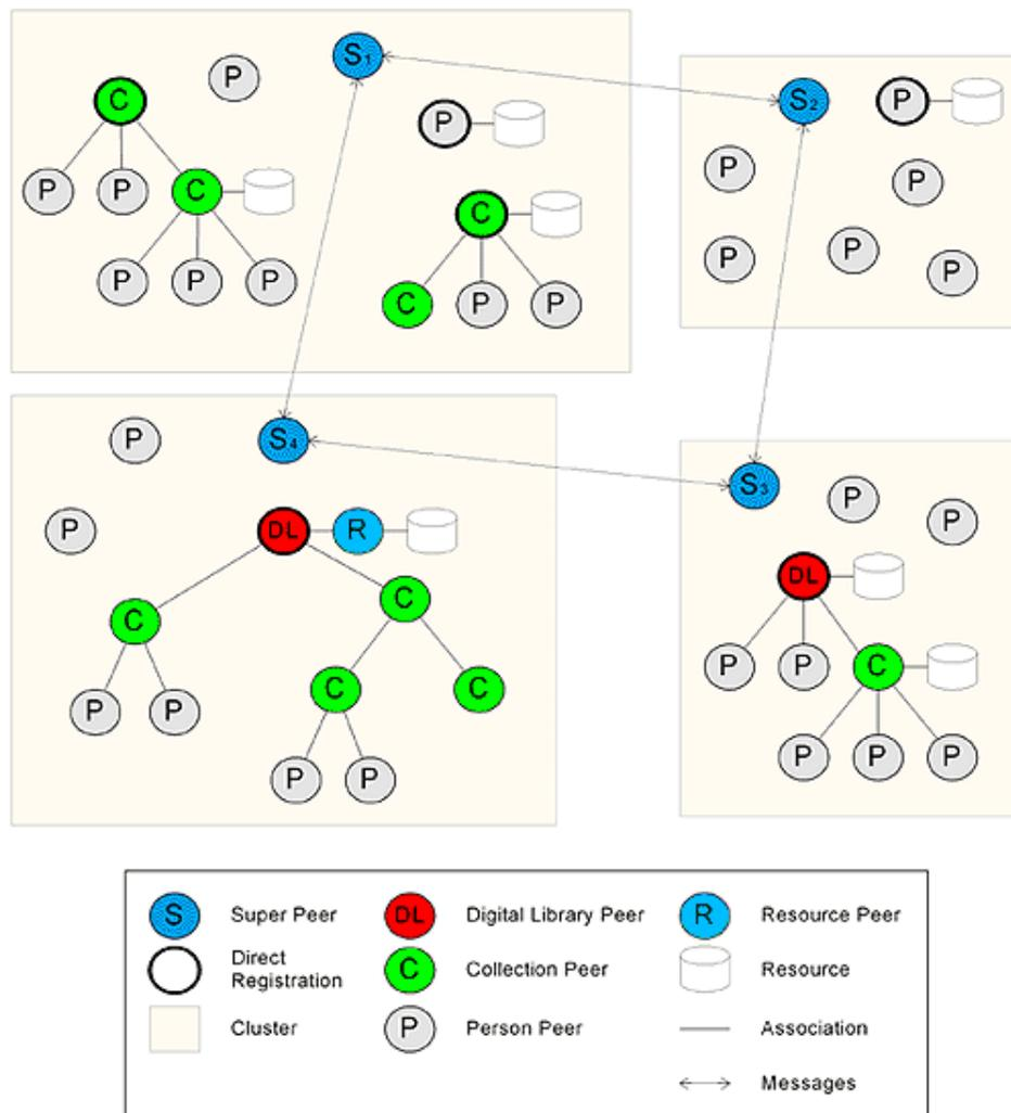
Figure 26 : A hierarchical super-peer network for distributed artefacts<sup>15</sup>
