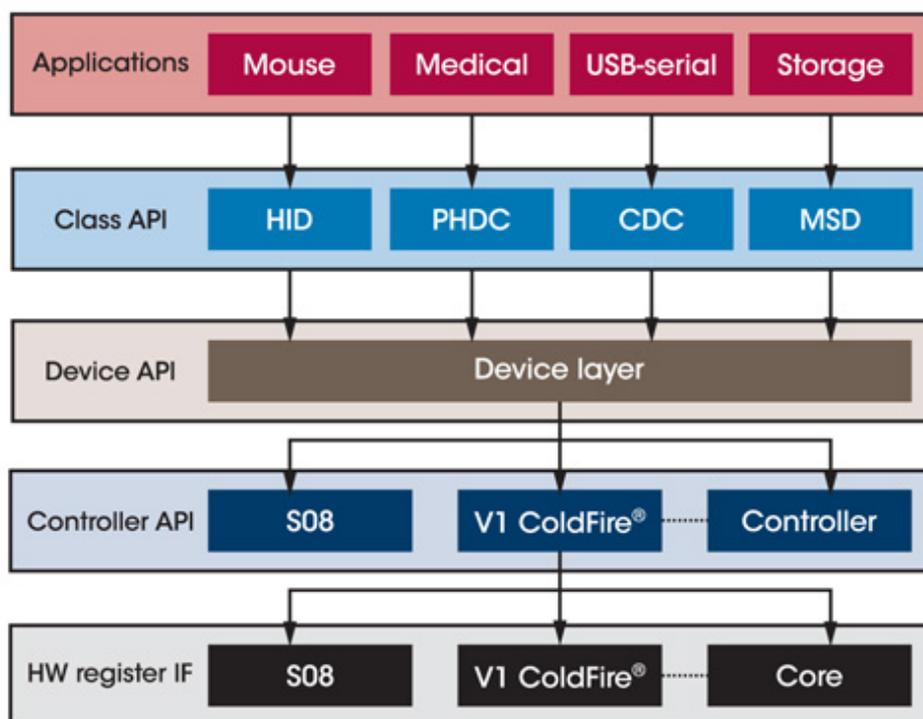
Figure 21 : Showing a block diagram of a USB stack with PHDC support.
