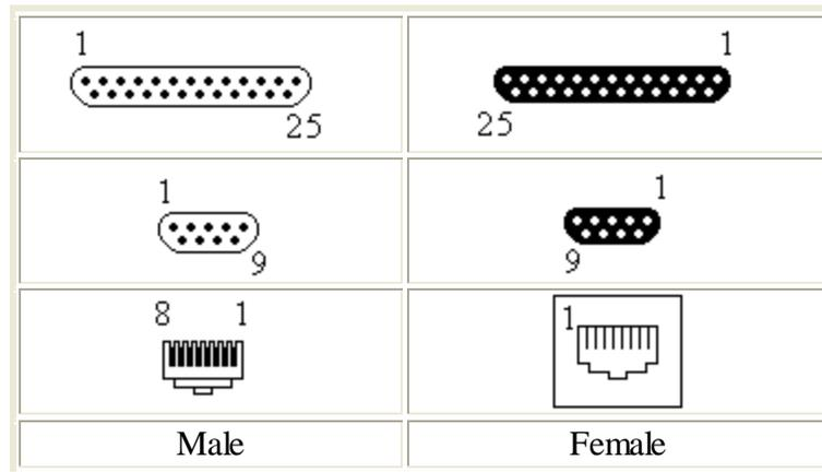
**Figure 19 : Types of RS-232 connectors**
