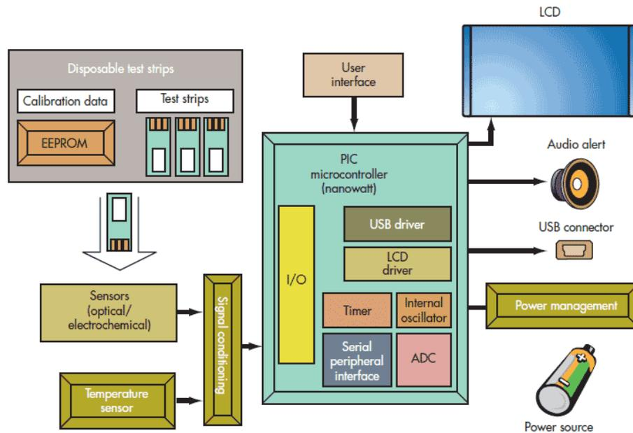
Figure 27 : Example of a home glucose meter circuit with microcontroller<sup>16</sup>.
