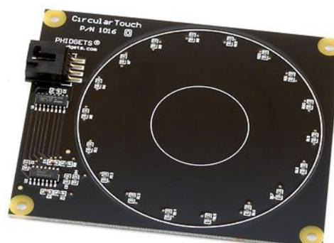
**Figure 32 : Phidget sensor that provides touch as input control.**
