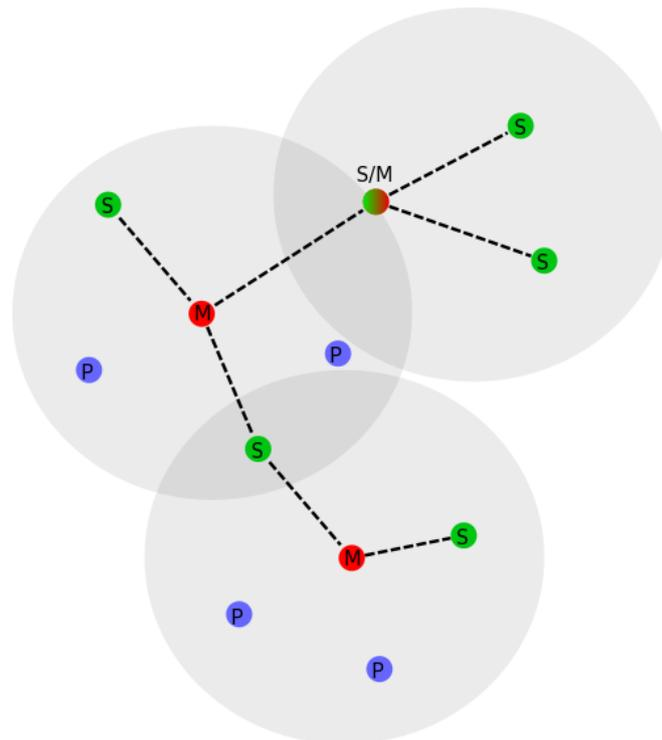
**Figure 3 : Example of Bluetooth network topology (M: Master, S: Slave, P; Parked)**
