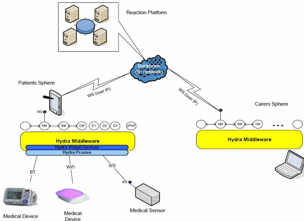
**Figure 35 : Incorporation of devices using the Hydra middleware.**
