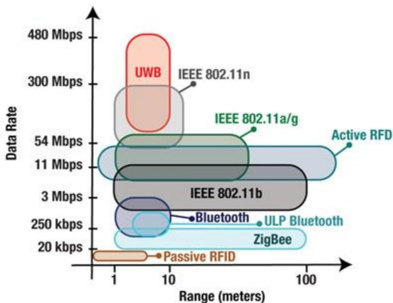
Figure 22 : Showing distribution of various communication protocols data rate and range<sup>12</sup>
