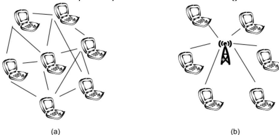
**Figure 12 : WLAN network topologies: (a) ad-hoc and (b) infrastructure**
