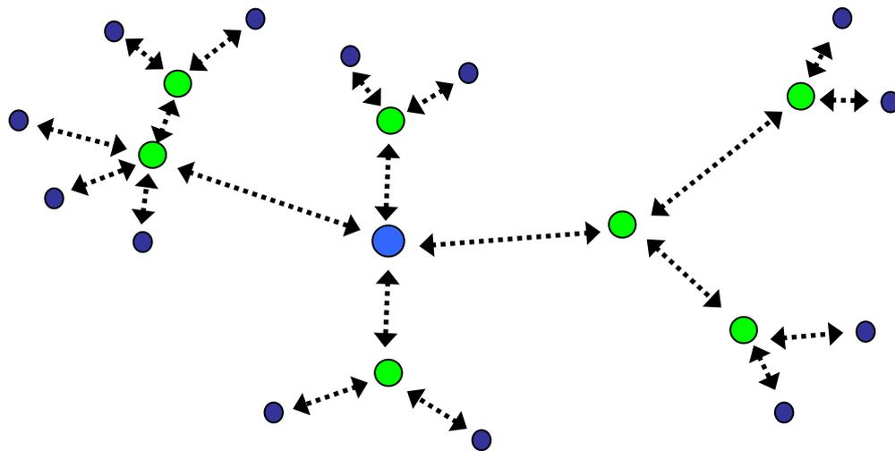
Figure 8 : ZigBee network topology
