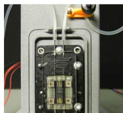
The non-invasive impedance spectroscopy sensor is already widely developed by SOLIANIS. However, since accuracy of non-invasive glucose sensors typically is somewhat lower compared to invasive methods, a second minimally invasive method was investigated by partner IMM who developed a prototype based on infrared absorption spectroscopy which has been tested in-vitro.
