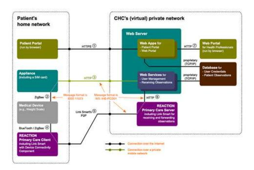
When the REACTION Primary Care Client application has been configured and deployed in the patient's home, the patient can simply turn on the PC and start taking measurements from his devices e.g. for blood glucose, blood pressure and weight. The results will automatically be sent to the clinical staff via a gateway, plugged into a wall socket.
